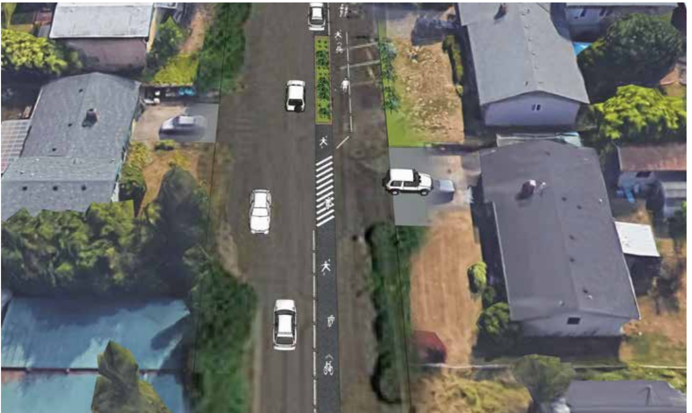
Below: Transitional street with curb stop protected pedestrian zone, driveway striping and planting buffer
